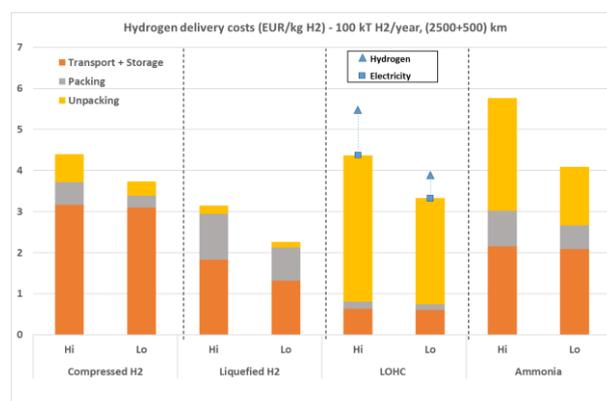
Figure 3 Hydrogen delivery costs for case B. Hi and Lo electricity prices for each carrier. Transport options involve a combination of shipping, train and truck.
