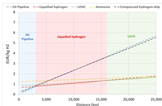
Figure 2 Hydrogen delivery costs for a simple (point to point) transport route, for 1 Mt H<sub>2</sub> and low electricity cost scenario.
