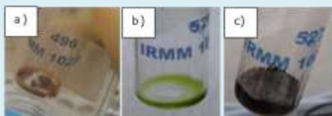
Figure 5. Appearance of CAB coated spike (a) before and (b,c) after reconditioning with H<sub>3</sub>PO<sub>4</sub>.
