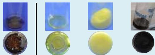
Figure 1. Flaked, unreliable LSD spikes (left) and different pathways that lead to improved integrity and stability (right – CAB + DOP, CMC, H<sub>3</sub>PO<sub>4</sub>)
