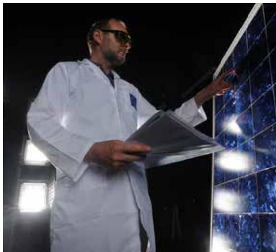
*The new Apollo large-area steady-state simulator opens the door to new measurements on advanced products as it provides full sunlight conditions over a 2mx2m test area for up to 8 hours.*
