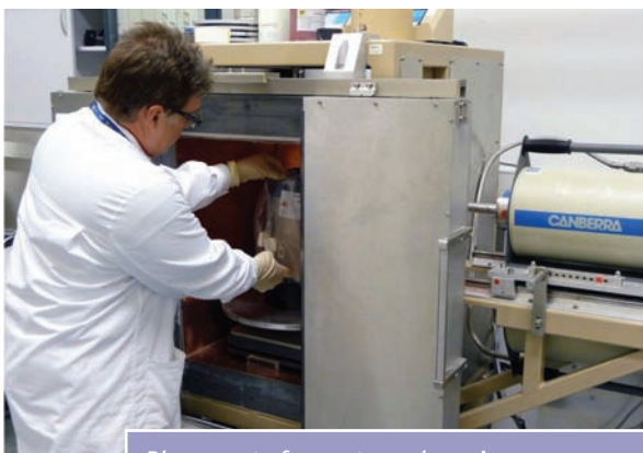
Placement of a waste package in a gamma measurement station and evaluation of the measurement results
