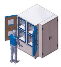
Twelve identical temperature chambers integrated into three cabinets, one shown on the left - BiA MTH 4.46 - for testing batteries were purchased in 2013 and 2016 (C112219). The system is equipped for providing controlled temperature independently inside each chamber.
