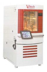
The climate chamber Vötsch VCS3 7060-5 for testing batteries will be purchased in 2013 (currently under procurement, the winning offer for Lot1 of C111682). The system is equipped for providing climate control i.e. controlling temperature and humidity inside the chamber.
