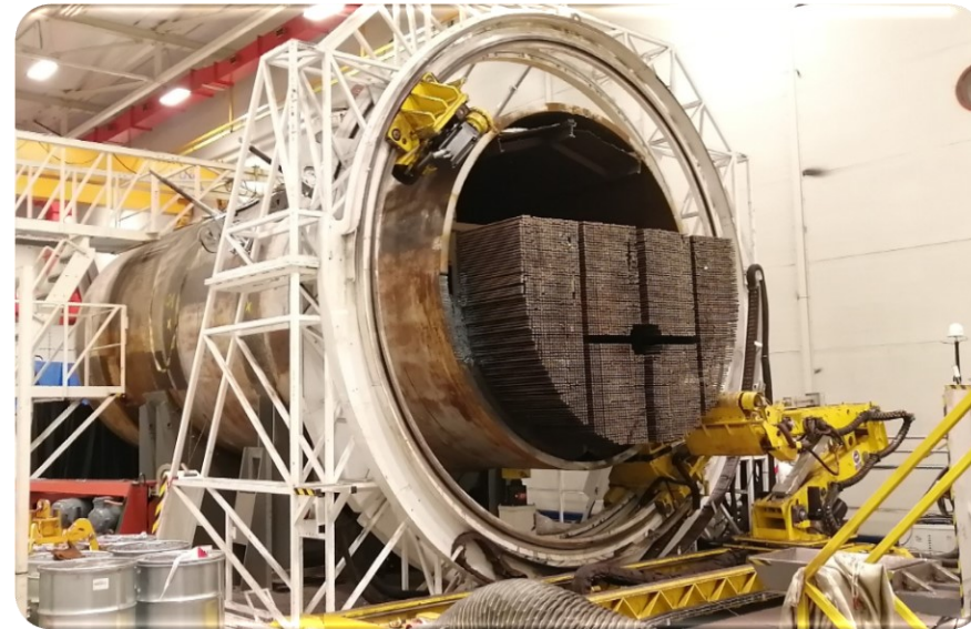
Turbine Hall – temporary storage & fragmentation in Dry-Cutting Workshop (DCW) in Turbine Hall
