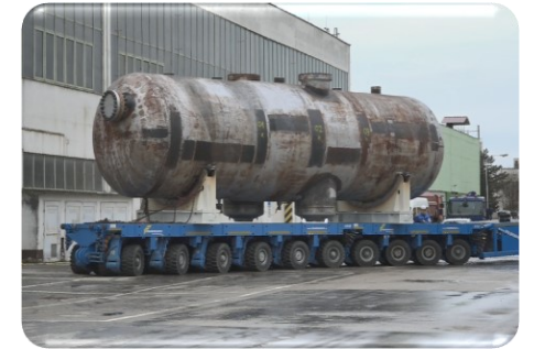
A special truck transported the individual SGs into the turbine hall
