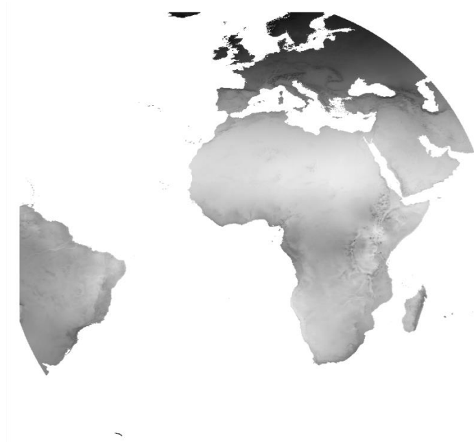
Figure 2 PV yield map 2005-2020, using SARA-2 irradiance data for the purpose of showing data completeness (lighter grey means higher yield in kWh/kWp)
