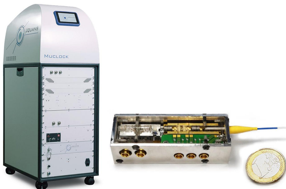
Figure 61 – A commercial cold-atom clock (left) and a prototype of an optical frequency standard based on two-photon transition in Rb (right). Note that in the latter the frequency comb necessary to translate the optical stabilised frequency into a microwave signal is not included [Strangfeld 2021]
