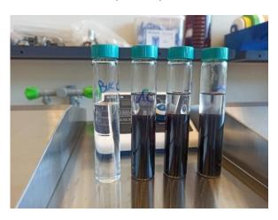
Sample A - After extraction with 15 ml hexane and addition of 2.5 ml ethanol for better phase separation
