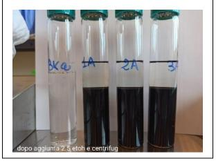
Additional examples – impact of time & shaking on the efficiency of the saponification a)- after 30 min at 60  $^{\circ}$ C – manual shaking at 15 min
