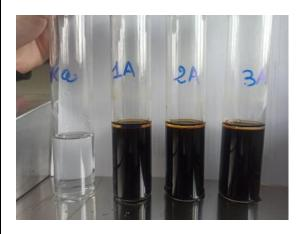
Sample C - After extraction with 15 ml hexane before addition of 2.5 ml ethanol
