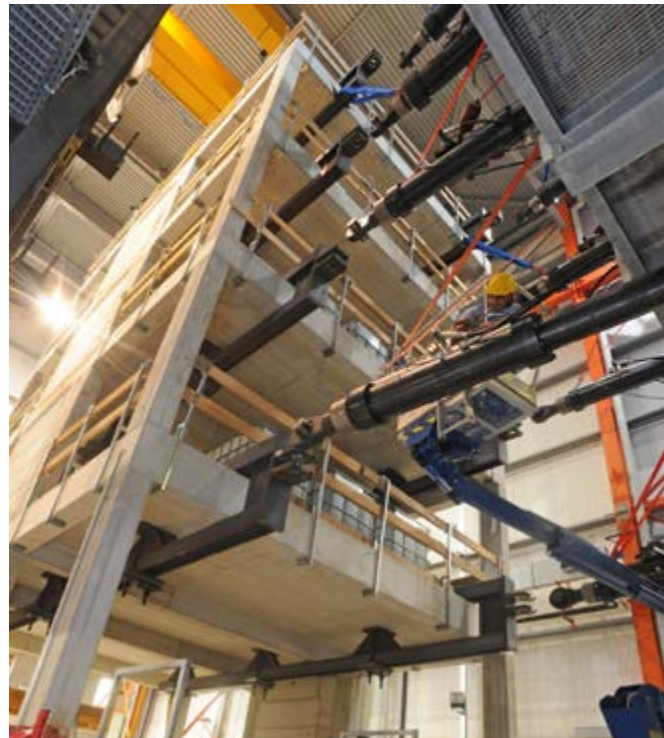
Setup of a large-scale structural test at the ELSA Laboratory: positioning and mounting of servo-hydraulic loading actuators.
