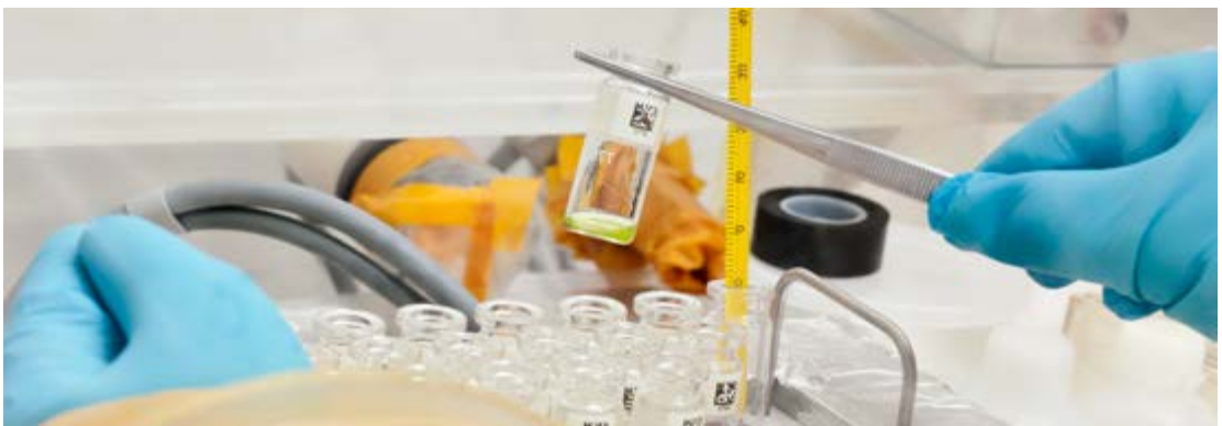
Evaporation of uranium plutonium large size dried spikes produced by the JRC in support of nuclear safeguards.
