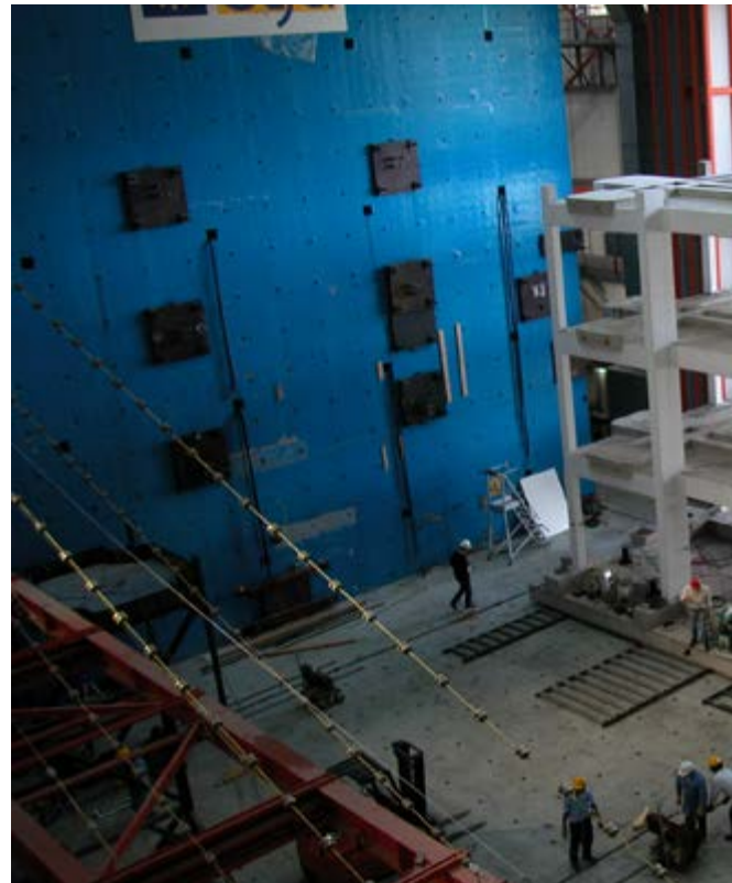
Reaction Wall of the European Laboratory for Structural Assessment at the JRC, Ispra.
