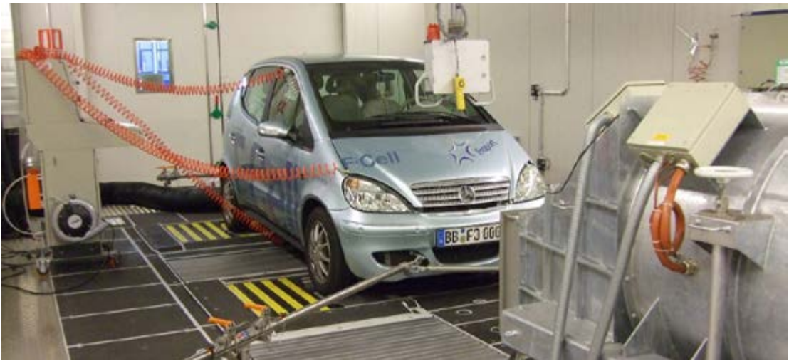
Emission test facility for light duty vehicles (passenger cars and light commercial vehicles). Energy efficiency test on a hydrogen fuel cell vehicle.
