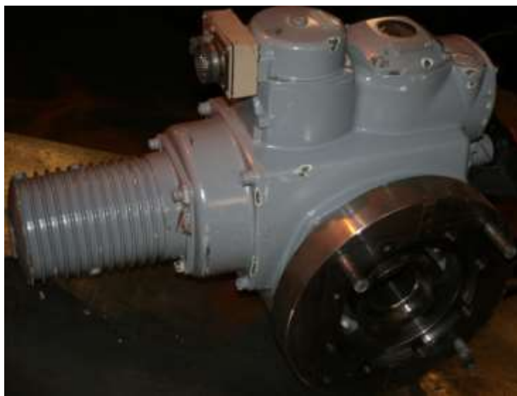
Figure 9. Valve servo actuator prepared for gamma-spectroscopy measurements.
