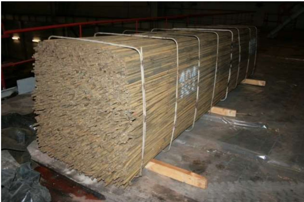
Figure 7. Example of tube pack prepared for gamma-spectroscopy measurements.
