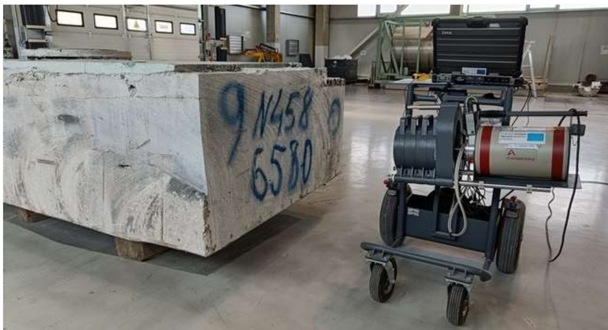
Figure 6. Example of mobile gamma-spectroscopy measurement system
