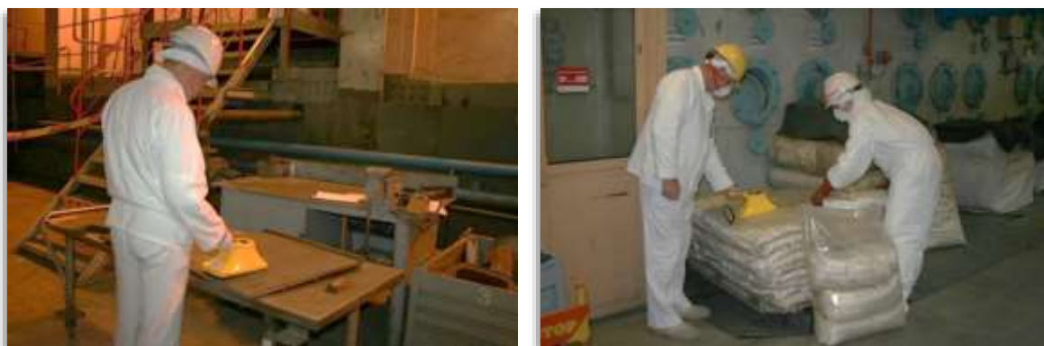
Figure 3. Surface \beta -contamination measurements.
