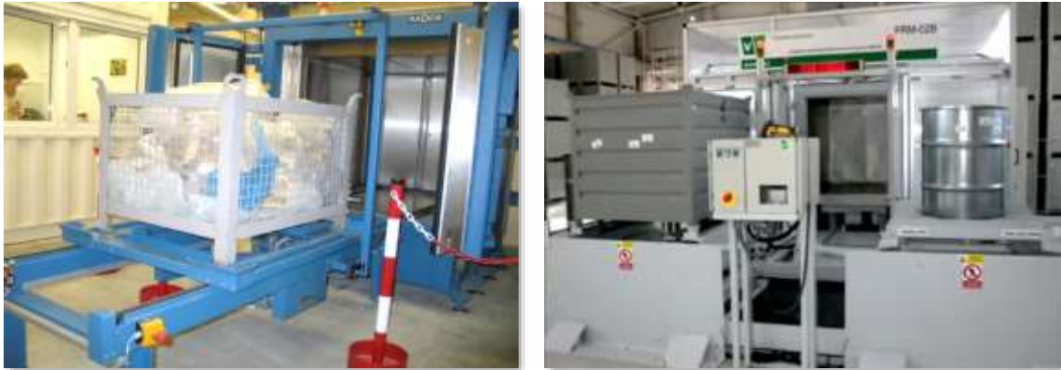
Figure 4. Examples of waste measurements in standard containers and drums.
