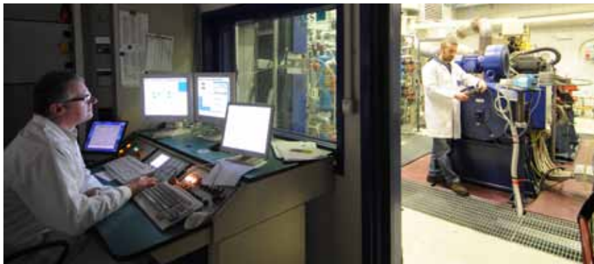
IES staff preparing a heavy duty diesel engine for emissions testing
