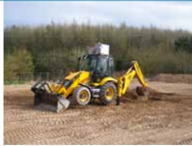
Use of Portable Emissions Measurement Systems (located in the boxes on the roof of the excavator) to monitor the exhaust emissions of non-road mobile machinery
