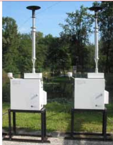
A sampling device developed and validated by the IES in Ispra for measuring carbonaceous aerosols.
