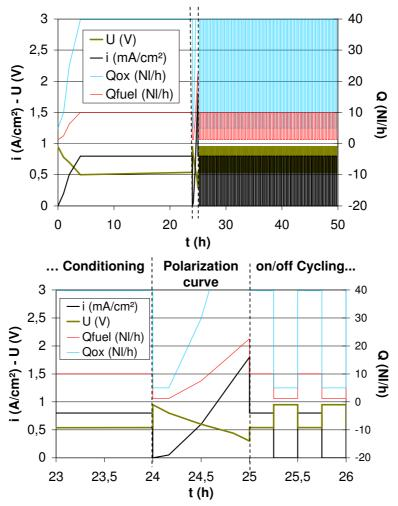
Figure 7.1: description of a on/off cycling accelerated ageing test (up: including start-up) and (down: detail with the end of the conditioning and the beginning of the cycling) where
