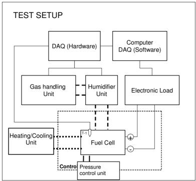
Figure 6.1: typical fuel cell test environment.
