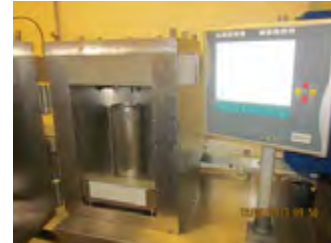
Picture of the UCMS showing the balance. 38 He-3 tubes are embedded in the walls. ID systems are placed over the container lid
