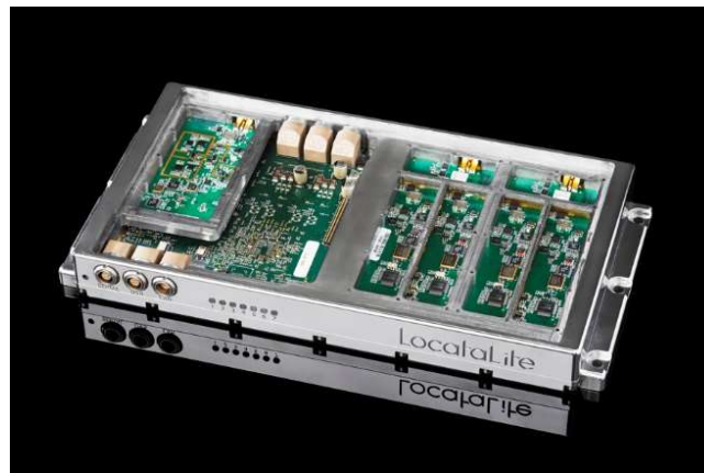
Figure 1-1: Locata Transmitter – LocataLite (with top cover removed)
