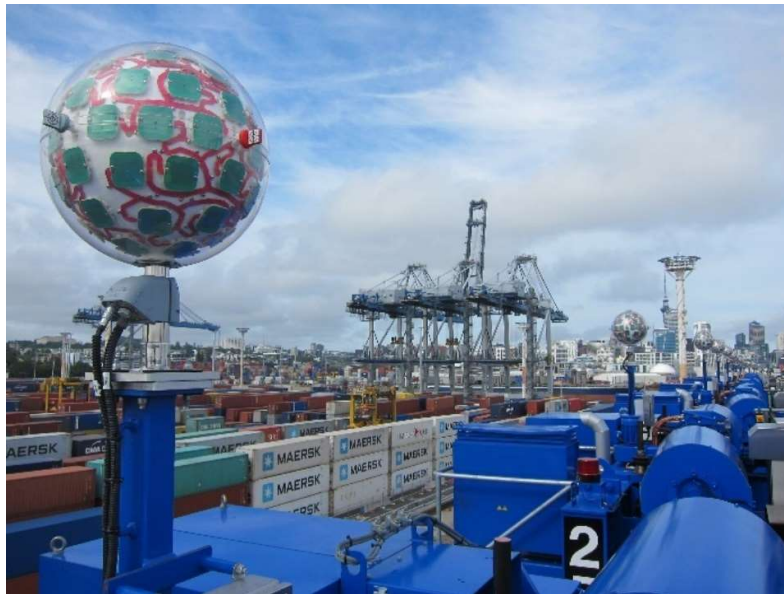
Figure 1-3: Locata V-Ray (“Orb”) Multipath Mitigation Antenna (a current production 60-element version shown)
