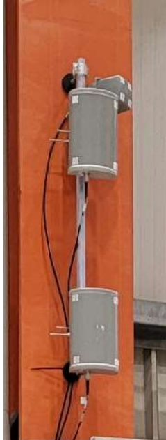
Figure 4-2: LocataLite with Indoor Wall (180° Coverage) Antennas
