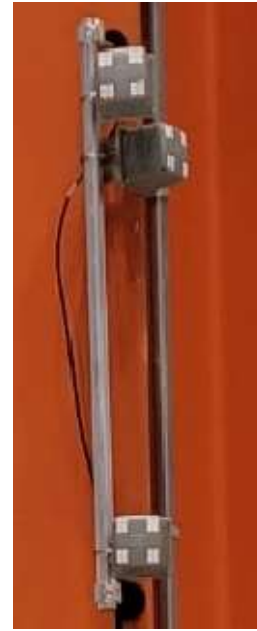
Figure 4-3: LocataLite with Indoor Corner (90° Coverage) Antennas
