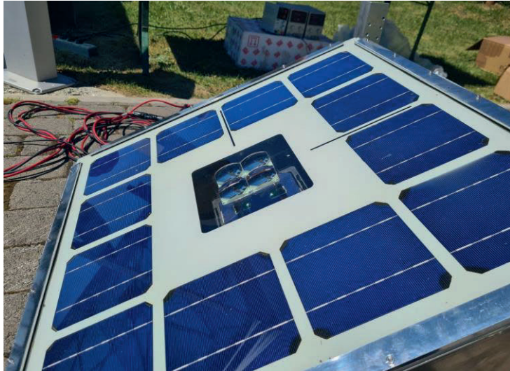
Figure 14: Front view of a functional unit of hybrid CPV / PV module with integrated solar tracking system based on SMA actuators, consisting of 4 lenses that focus the light on 4 high-efficiency CPV cells positioned on a moving frame that moves parallel to the p
