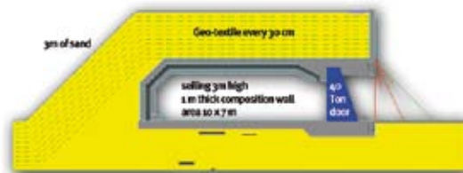
Cross section of the bunker
