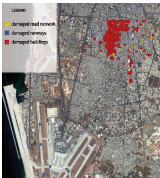
Damage assessment has been done using photo-interpretation of post-conflict Ikonos satellite imagery over Beirut recorded on 19 August, 2006
