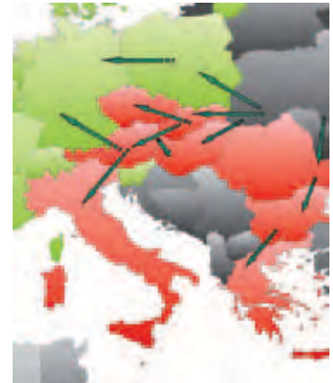
The GEMFLOW gas model simulates the exchange of gas between Member States in the event of a gas disruption, taking into account demand, production, Liquefied Natural Gas (LNG) as well as storage measures.
