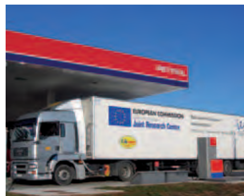
Truck equipped with portable emissions measurement systems on a long-distance test between Ispra and Barcelona.
