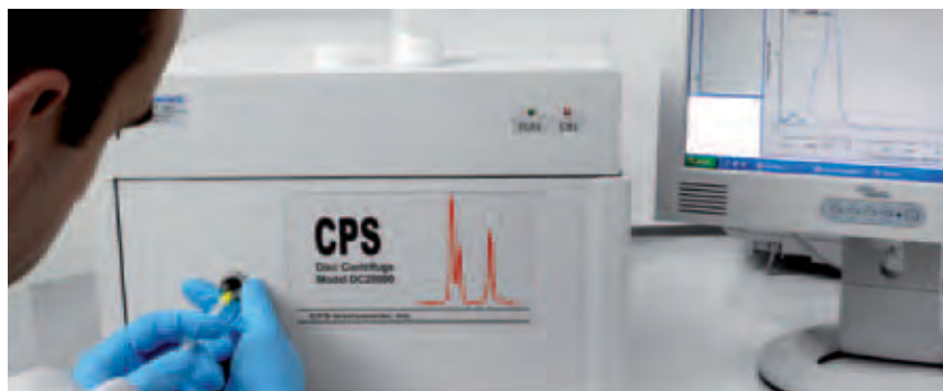
Centrifugal liquid sedimentation instrument to measure the size distribution of nanoparticles in a suspension.
