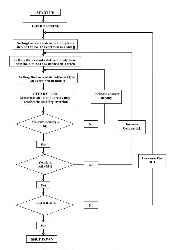
Figure 7.2: Test procedure overview
