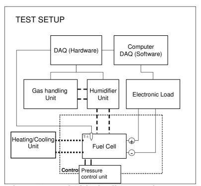
Figure 6.1: typical fuel cell test environment.
