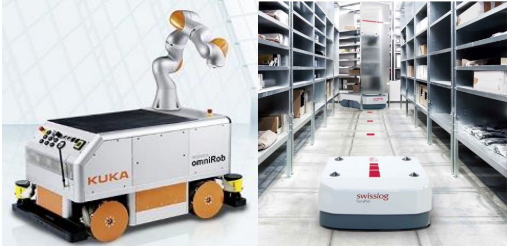
Figure 5: Two examples of automated guided vehicles. The KUKA omniRob (left) with a modular design that can include a mechanical arm. The Swisslog/KUKA CarryPick (right) moves shelves around a warehouse and brings them to human workers, for them to pick and package the product from the shelf.
