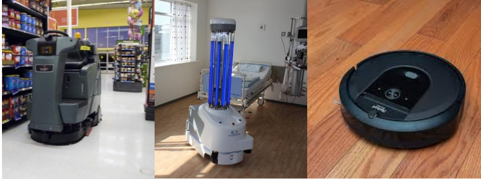
Figure 6: The Auto-C by BrainOS (left) is used by Wal-Mart to clean floors in its stores. The UVD robots (centre) clean and disinfect hospital rooms. The Roomba (right) is a best-selling personal cleaning robot for domestic use.
