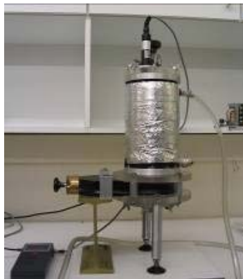
Fig. 2: Set-up of the aerosol deposition chamber
