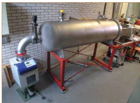
Full-scale permeation test at JRC-IE's fuel storage testing facilities
