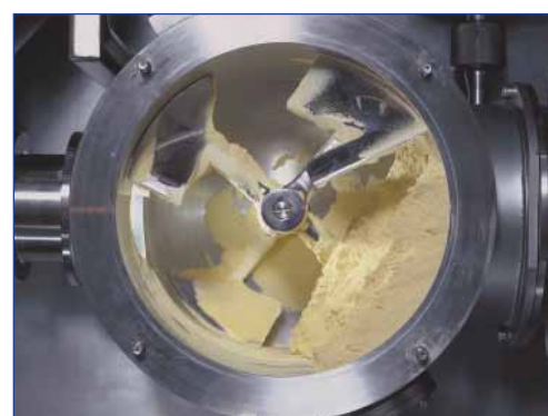
A dry mixing technique is applied for processing GMO reference materials to avoid DNA degradation
