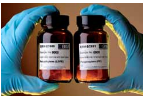
Certified reference materials were developed to help analytical laboratories better detect two classes of flame retardants banned under the RoHS Directive.
