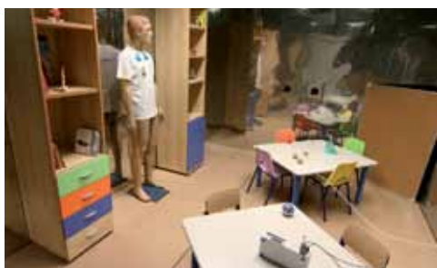
The Indoortron laboratory measures indoor pollution. In the 30m 3 volume walk-in chamber which has controlled temperature, relative humidity, air quality and air exchange rate, the sources of indoor pollution by volatile organic compounds and their impact on our health and comfort are studied.
