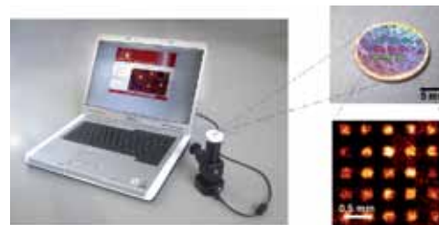
Prototype of the Multiplexing Nanoplasmonic Sensor developed by Plasmore. The prototype of the biochip is a glass disk consisting of a nanostructured surface and a protein microarray.
