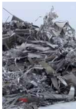
For ferrous metals such as iron and steel, waste would have to contain less than 2% of non-metallic elements to qualify.
