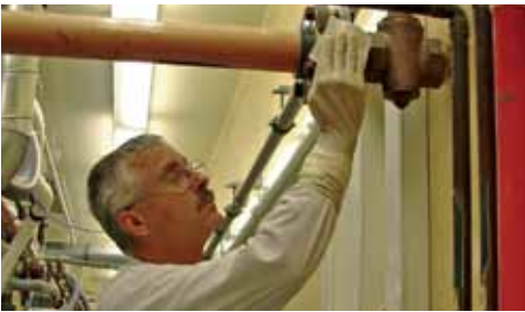
Swipe sampling technique used to collect dust at a nuclear facility.
