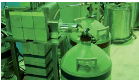
In the framework of the TACIS project, the nuclear material accountancy measurement system at the RT-1 reprocessing facility in Mayak (Russia) was upgraded. The picture shows a Hybrid K-Edge instrument with sample changer, suitable for measuring the U and Pu concentration in spent fuel solutions. The instrument is installed in a hot cell.
