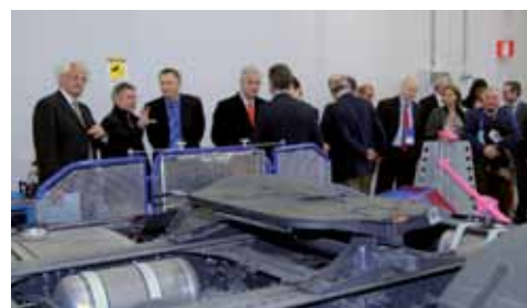
VELA-7 can host vehicles weighing up to 30 tons, and 12 metres long, simulating wind drag, tyre/road friction as well as full drive cycles.
