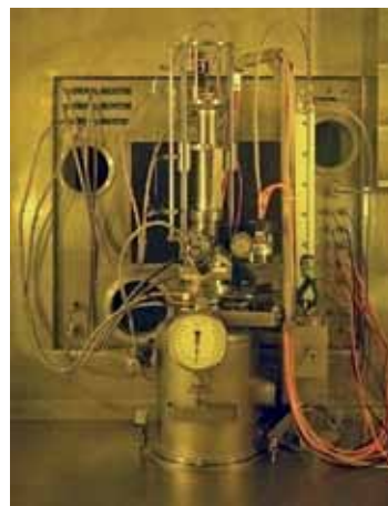
The new Küfa device, a furnace in which certain off-normal conditions can be simulated, installed in the JRC-ITU Hot Cells unit.
