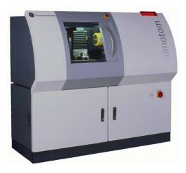
The X-Ray computed tomography system Phoenix nanotom s was purchased in 2011 (C108733) and allows for X-ray computed tomography (CT) i.e. 3D imaging of a wide variety of materials.
