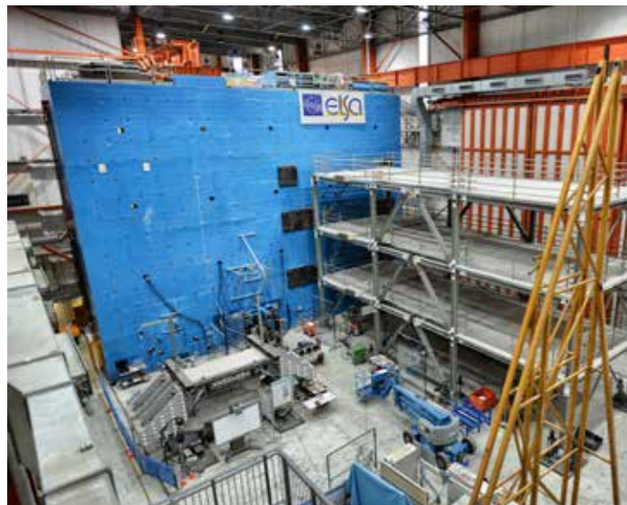
The JRC's European Laboratory for Structural Assessment (ELSA) is equipped with one of the three largest reaction walls in the world to test the vulnerability of buildings against earthquakes.
