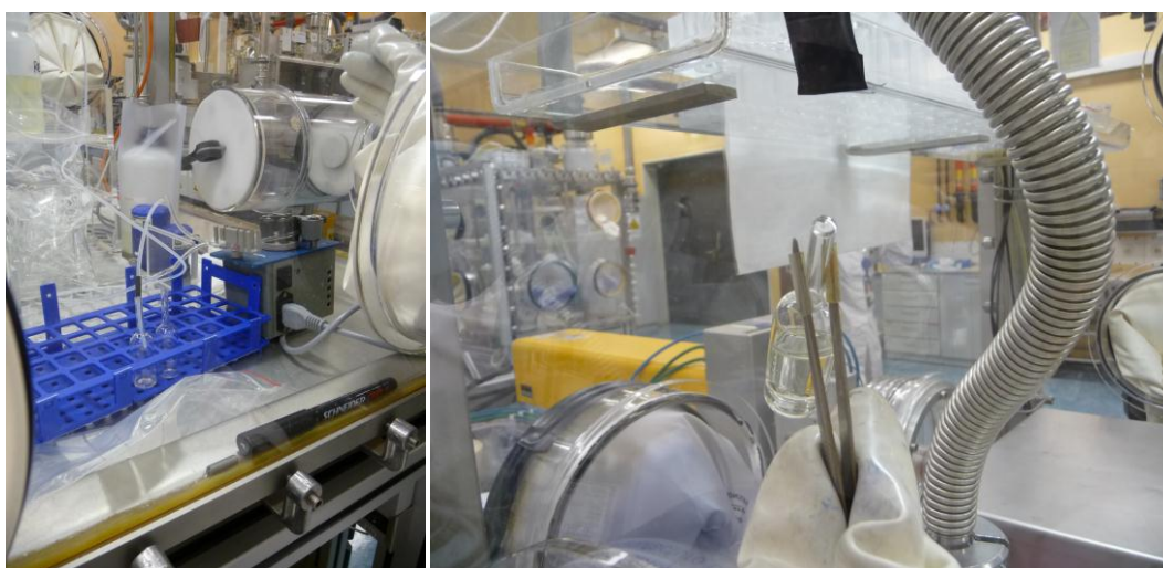
Figure 1: Dispensing of a REIMEP-17B sample with a peristaltic pump inside the glove box (left) and sealing of an ampoule (right) at JRC-ITU Karlsruhe.
