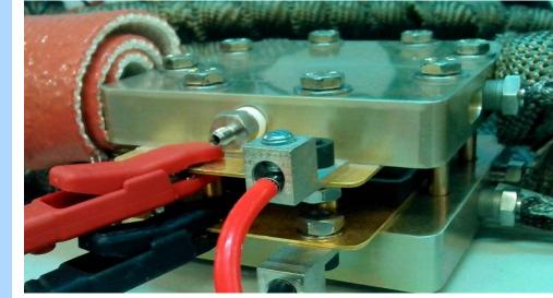
Fuel cells are often described as a continuously operating battery. They produce electricity via an electrochemical process: hydrogen from a hydrogen-containing fuel is combined with oxygen. Because of their high conversion efficiency, reduced pollution and low noise, fuel cells in the future can play a major role in energy conversion, and can partly substitute current power generation technologies in many end use sectors.
