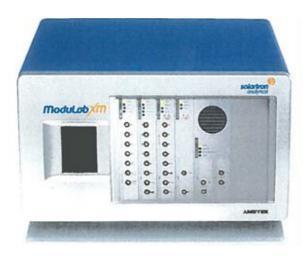
The system comprises of two main control modules: the potentiostat/galvanostat (XM PSTAT 1 Ms/s) and the FRA (XM FRA 1 MHz/300 KHz) module.
