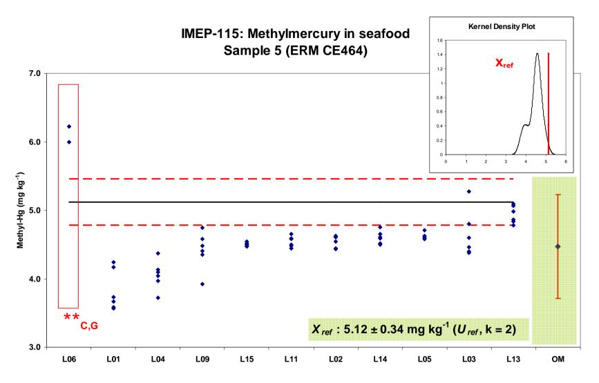
This plot shows all measurement results. The solid line refers to the  $X_{ref}$ . The dotted line the boundaries of  $X_{ref}$  ( $X_{ref} \pm U_{ref}$ ), OM refers to the overall mean ( $X_{Obs} \pm 2S_R$ ). Identified laboratory was considered outlier.
