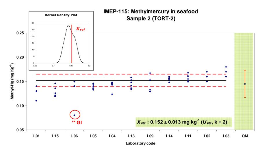
This plot shows all measurement results. The solid line refers to the  $X_{ref}$ . The dotted line the boundaries of  $X_{ref}$  ( $X_{ref} \pm U_{ref}$ ), OM refers to the overall mean ( $X_{Obs} \pm 2S_R$ ). Identified replicate was considered outlier.
