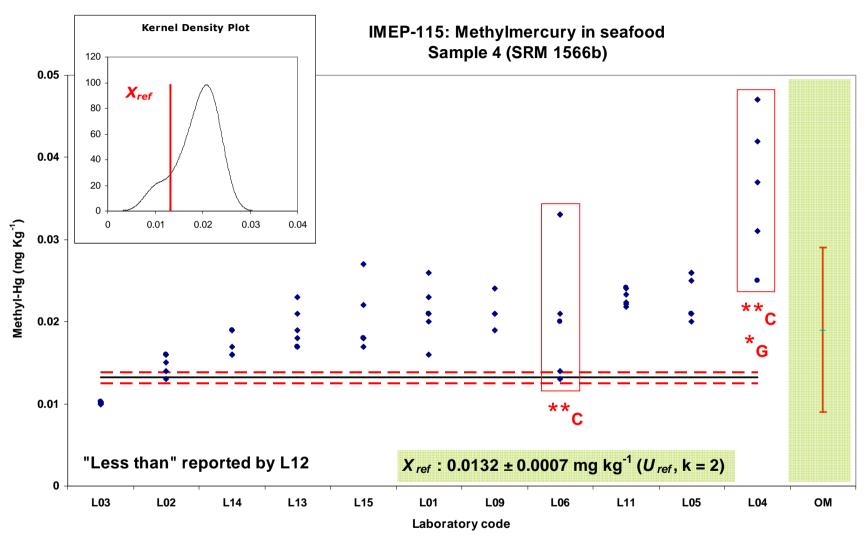
This plot shows all measurement results. The solid line refers to the  $X_{ref}$ . The dotted line the boundaries of  $X_{ref}$  ( $X_{ref} \pm U_{ref}$ ), OM refers to the overall mean ( $X_{Obs} \pm 2S_R$ ). Identified laboratories were considered outliers.
