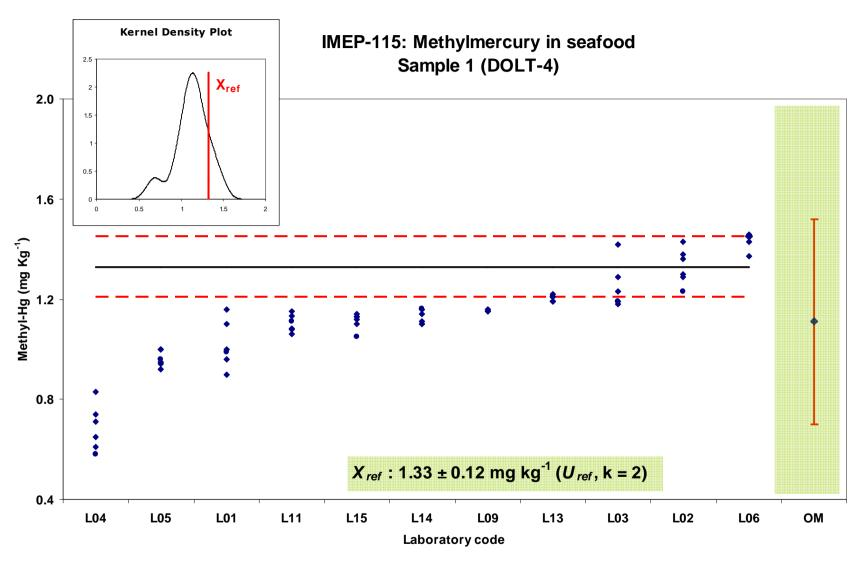
This plot shows all measurement results. The solid line refers to the  $X_{ref}$ . The dotted line the boundaries of  $X_{ref}$  ( $X_{ref} \pm U_{ref}$ ), OM refers to the overall mean ( $X_{Obs} \pm 2S_R$ )
