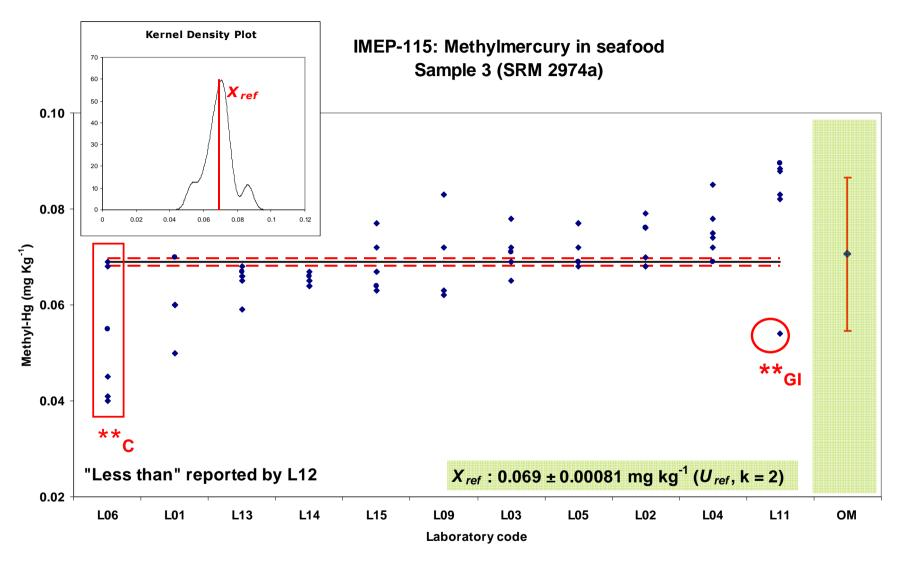
This plot shows all measurement results. The solid line refers to the  $X_{ref}$ . The dotted line the boundaries of  $X_{ref}$  ( $X_{ref} \pm U_{ref}$ ), OM refers to the overall mean ( $X_{Obs} \pm 2S_R$ ). Identified laboratory and replicate were considered outliers.
