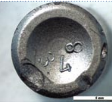
One of the uranium fuel pellets seized in Lauenförde (Germany). The pellet shows mechanical defects and markings on the top and on the bottom
