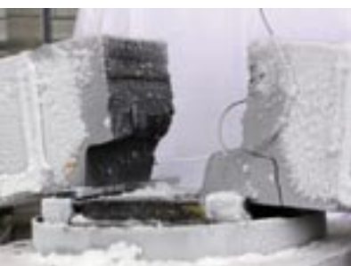
Structural integrity tests on reactor materials with simulated sub-surface flaws
