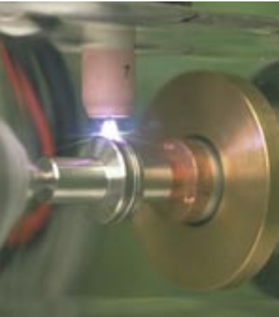
Welding Re-226 capsule for irradiation in a cyclotron to produce Ac-225
