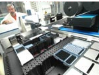
Automated testing facilities for in vitro cell-based toxicity assays
