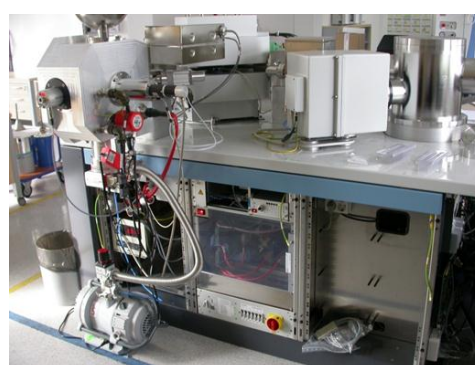
Measurement of U and/or Pu isotopic Ratios by Mass Spectrometry using new modified total evaporation method developed by JRC
