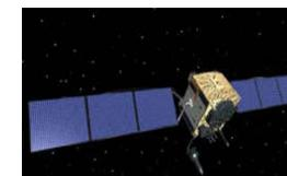
**12 operational GPS Block IIF sat (L1/L5)**
