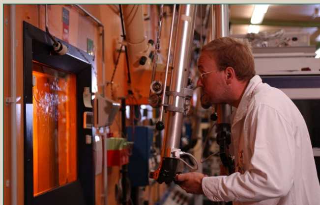
Hot cells facility for the analysis of spent fuel material.
