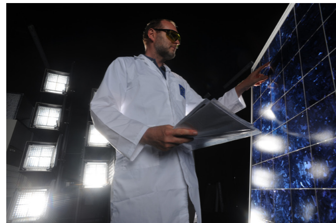
ESTI's new large-area steady state simulator opens a range of possibilities for studying the electrical performance of new module technologies with long response times.
