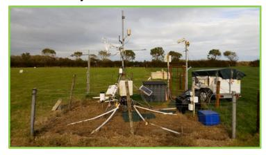
Integrates high frequency field scale N<sub>2</sub>O fluxes over a large area and multiple sources ©
