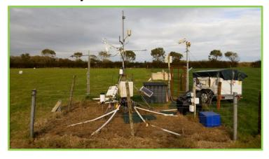
Integrates high frequency field scale N₂O fluxes over a large area and multiple sources ☺
