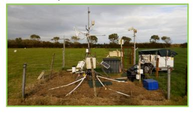
Integrates high frequency field scale N₂O fluxes over a large area and multiple sources <sup>©</sup>
