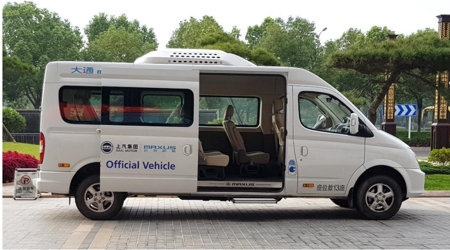
SAIC Maxus FCV 80 Van with 100 kW e propulsion power
